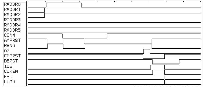
Figure 6. Operation using the correlator. Horizontal scale is 4  $\mu$ s per tick mark.
