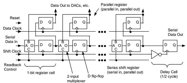
Figure 1. Architecture of serial data register.
