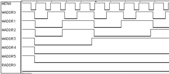
Figure 5. Writing to the AMU. Horizontal scale is 100 ns per tick mark.
