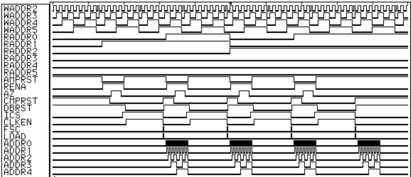
Figure 7. Pipeline operation showing four conversions. Setup is performed during data readout. Time scale is 5  $\mu$ s per tick mark.
