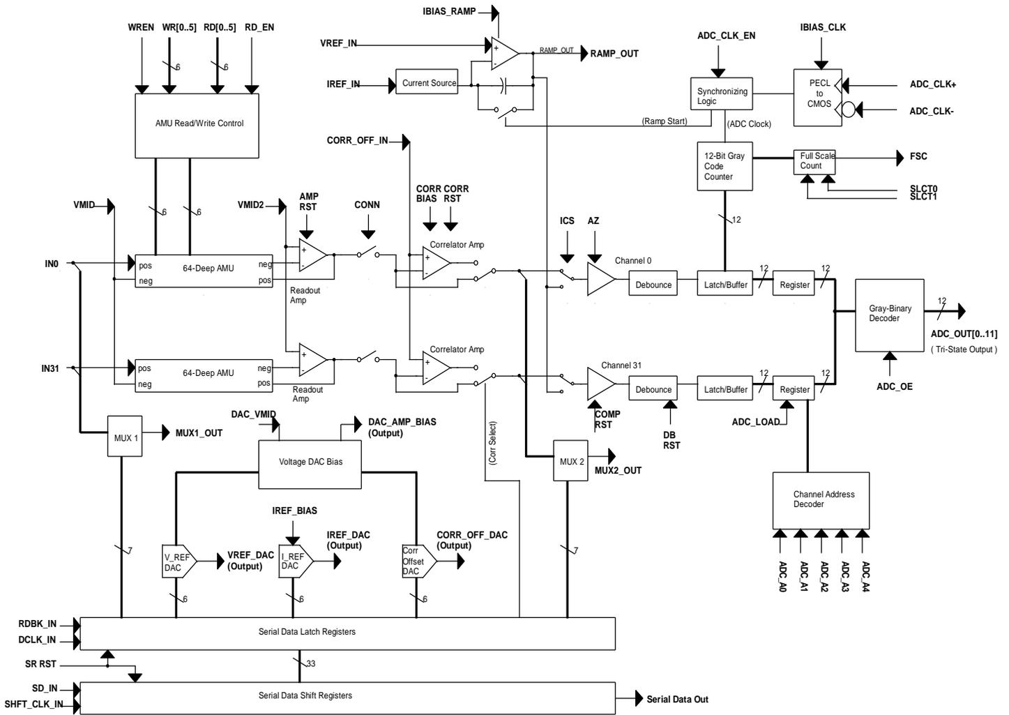
Figure 2. Block Diagram of AMU-ADC.
