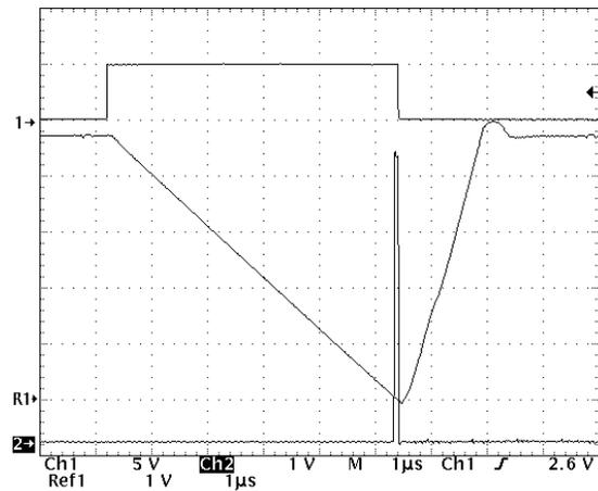
Figure 4. Typical adjustment of Ramp and FSC. Top trace (1) is ADC\_CLK\_EN at 5 V/div., middle trace (R1) is the Ramp at 1 V/div., and bottom trace (2) is FSC at 1 V/div. The horizontal scale is 1  $\mu$ s/div. The arrows on the left edge indicate the GND positions.
