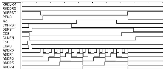
Figure 3. Timing for the ADC section. Horizontal scale is 0.5  $\mu$ s per tick mark.
